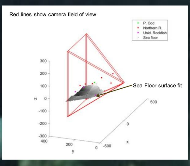
Height off the seafloor was determined by projecting a 3-D bottom profile onto the image
