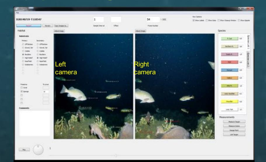
Used Sebastes stereo analysis software (Williams & Towler) Fish identified, measured, and counted in each image pair
