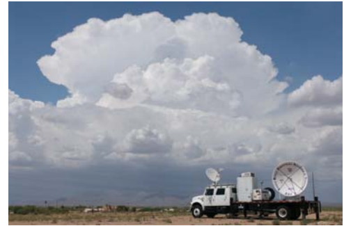
A SMART-R scanned this thunderstorm to provide precipitation data for a flash flood study in Phoenix, AZ during the summer monsoon season.
