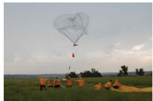
Techniques for launching balloons in high winds were developed at NSSL, allowing researchers to take upper-air soundings near thunderstorms.
