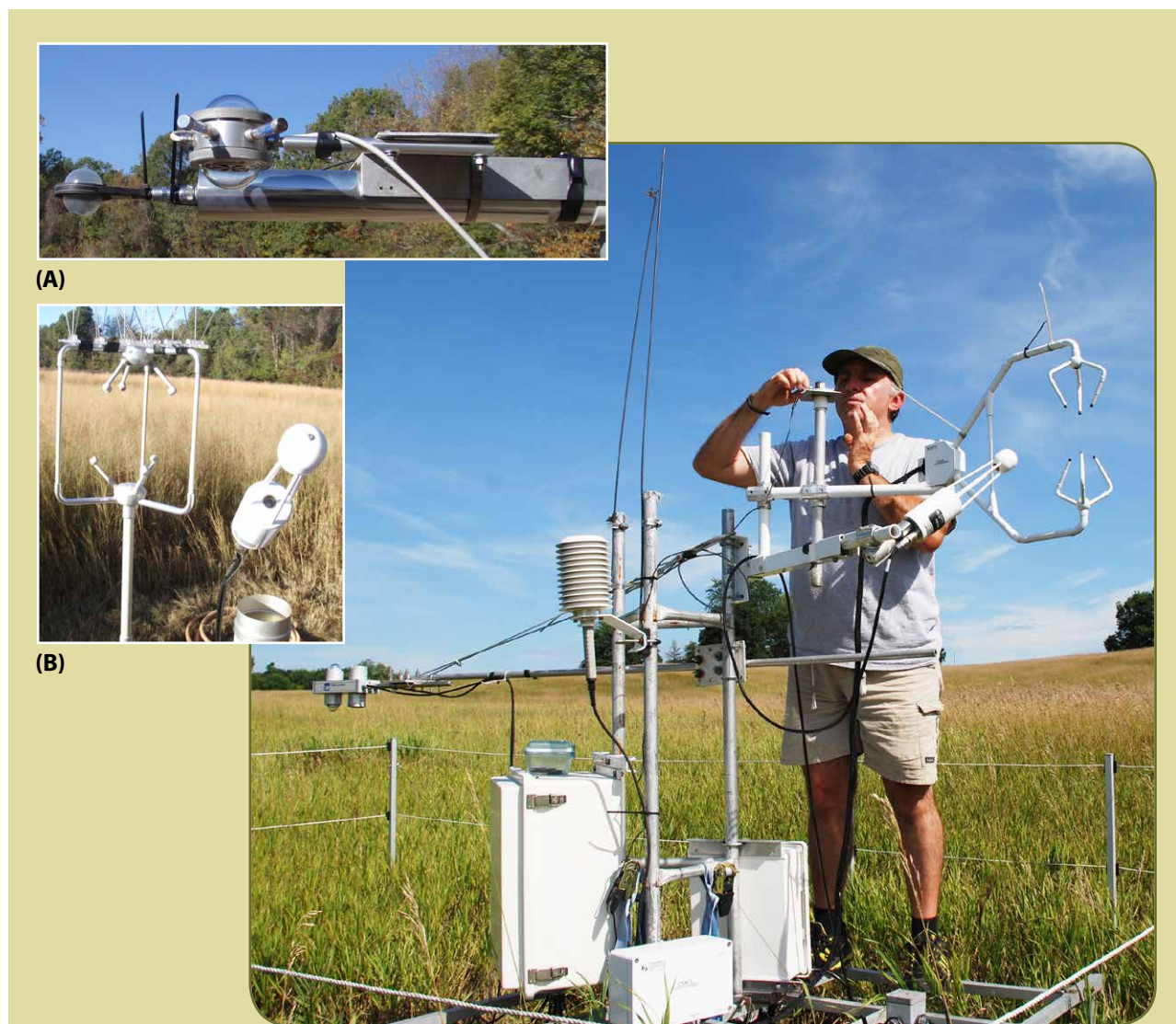
Fig. 10. Flux Tower Measurements. Researcher checks instrumentation on a carbon dioxide flux tower in a switchgrass field in Michigan. [Image courtesy B. Zenone, Michigan State University] (Inset A) Radiometers mounted on an eddy flux tower above a switchgrass field in Tennessee. (Inset B) Sonic anemometer and gas analyzer mounted on an eddy covariance tower measuring fluxes of energy, water, and carbon dioxide in a switchgrass field in Tennessee. [Inset images A and B courtesy T. Martin, Argonne National Laboratory]
