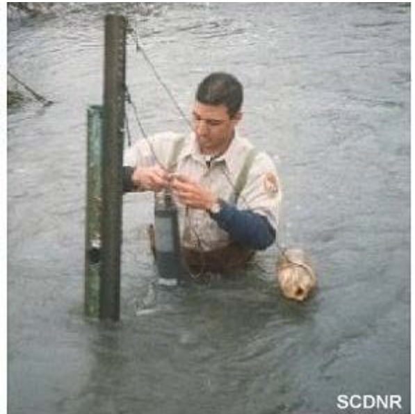
Deploying water quality monitoring instrumentation
