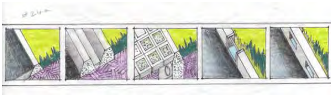
Figure 34-1. Eliminate curb and gutter – edge options
