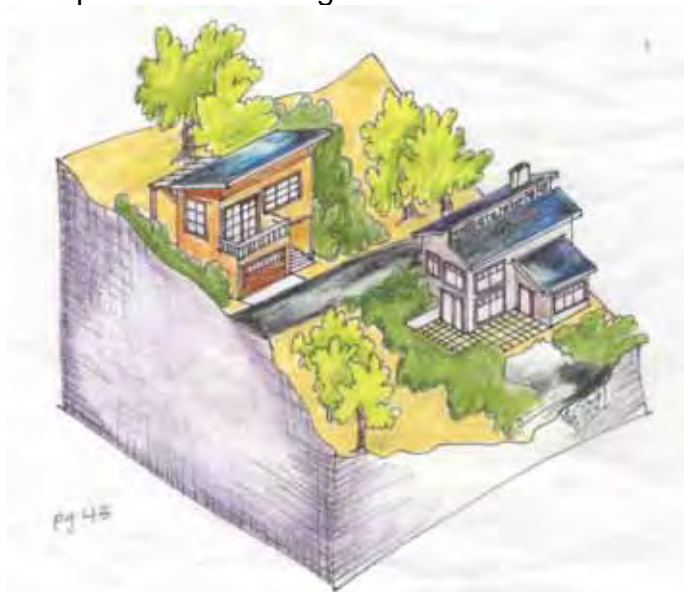
Figure 7-1. Fit development to natural gradient
