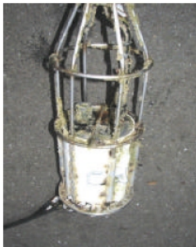
Figure 1: photograph of METOCEAN drifter 52197 in December 2005, roughly one week after its recovery during the CONGAS2 cruise. The subsurface sensor area is shown with noticeable algal fouling near the sensors.
