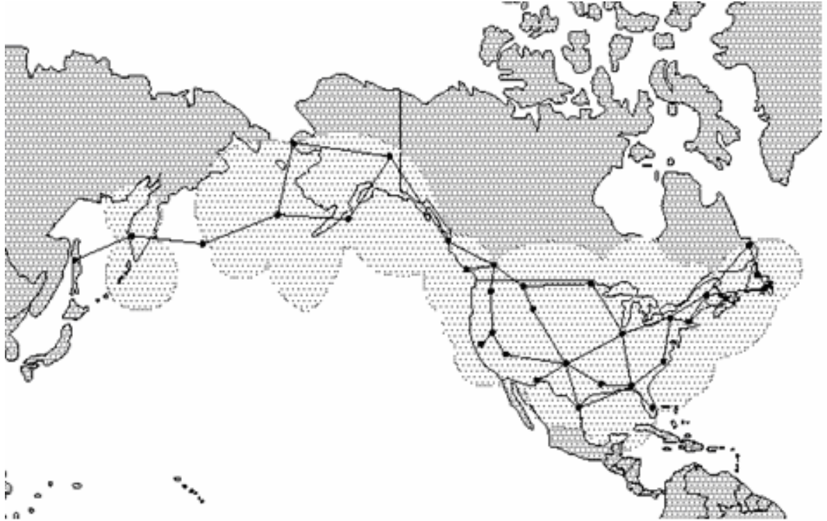
Figure B-8. Coverage Provided by U.S. or Supported Loran-C Station
