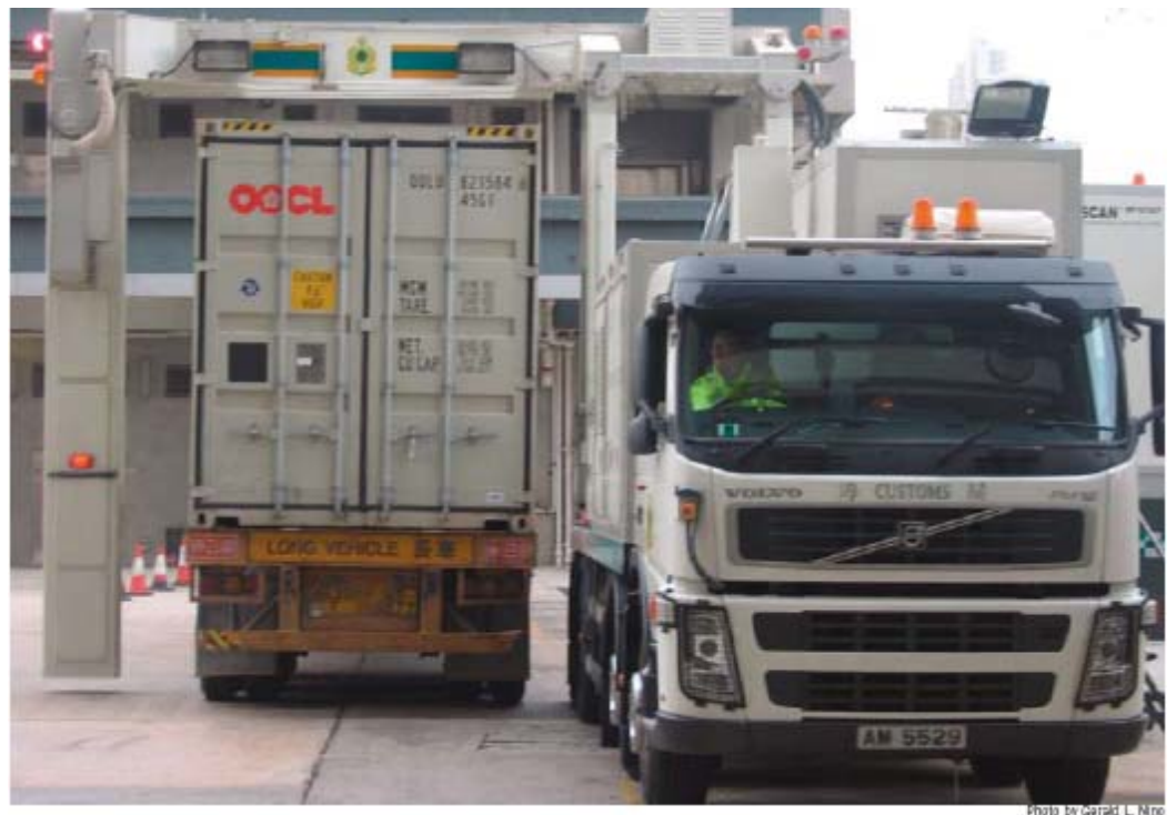
Figure 4: Radiation Detection Equipment at a Foreign Port
