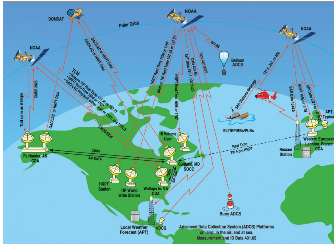
NOAA KLMN-N Prime Spacecraft Communications Radio Frequency (RF) Links (frequencies are in MHz)
