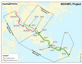
Improvements to the existing NFL project include levee and floodwall improvements, as well as fronting protection at pumping stations.
