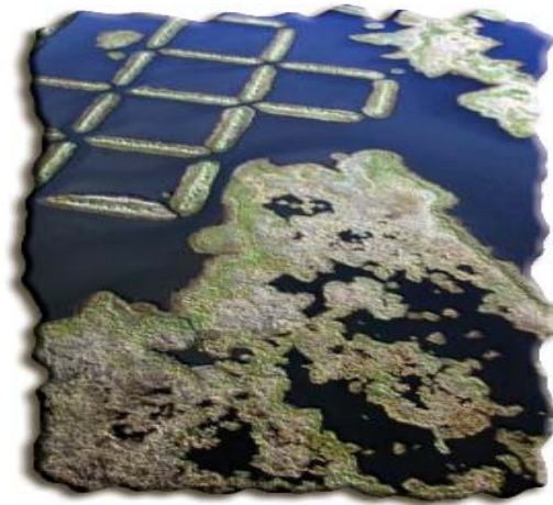
Open cells of earthen material at Brown Lake create sediment traps to rebuild marsh.
