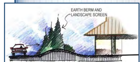
Fig. 9.18 – Landscape and Berms Buffer Air and Noise Pollution
