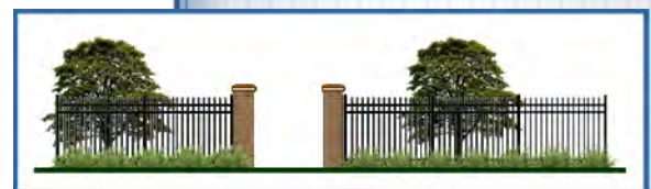
Fig 6.13 – Typical Black Aluminum Fencing and Brick Columns
