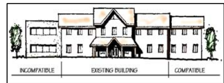
Fig. ES.42 – An illustration comparing compatible and incompatible additions.
