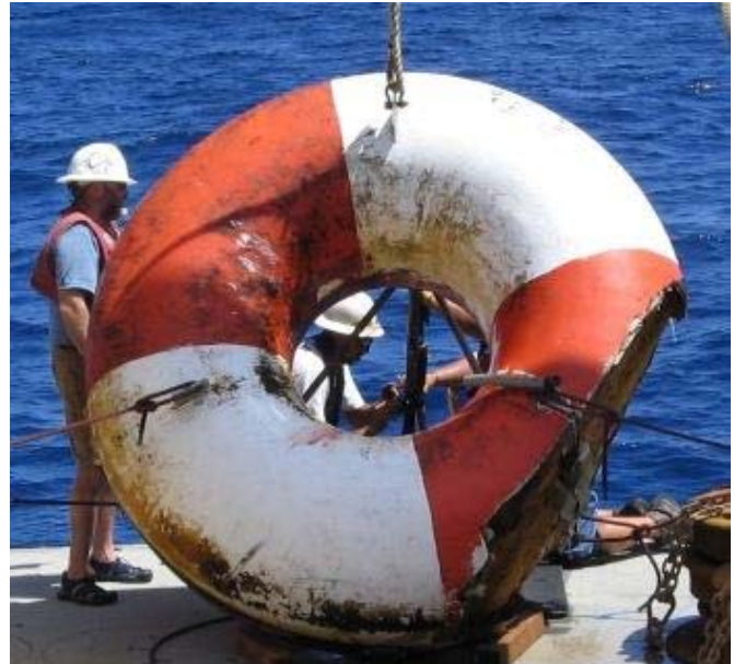
Figure 6 TAO buoy hull damage due to vessel collision
