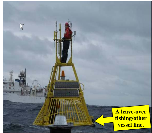
Figure 3 NDBC WxOP buoy vandalism: fishing activity
