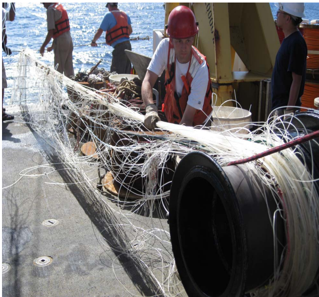
Figure 8 TAO buoy vandalism: long-line
