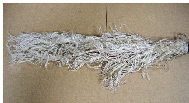
Figure 10 Tsunameter buoy vandalism: mooring line cut
