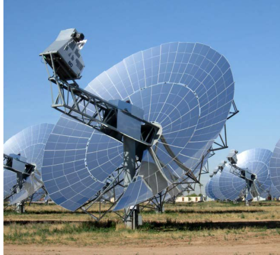
Figure A18. 25 kW dish/Stirling engine system made by Tessera Solar. Photo from NREL
