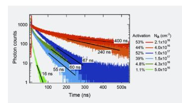
Time-correlated single-photon counting decay curves showing lifetime of photo-excited electrons in the research team's bulk CdTe as a function of hole density and activation levels, which are each two to three orders of magnitude better than those in traditional CdTe solar devices. Illustration by NREL.
