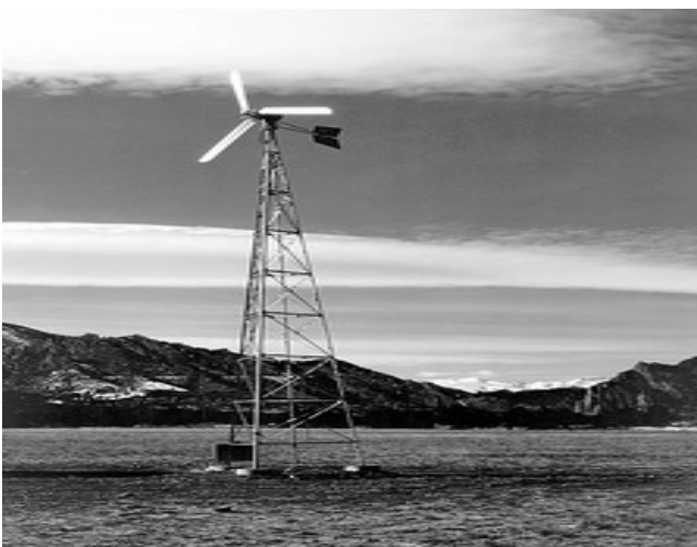
The Dunlite turbine, with 3 blades and a 12-foot rotor diameter, was tested at Rocky Flats. (circa 1977)
