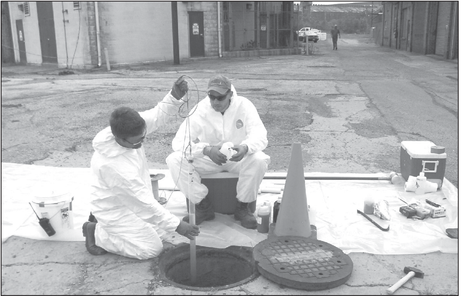
Workers do sewer water sampling at Harshaw Chemical Company in Cleveland during the remedial investigation.
