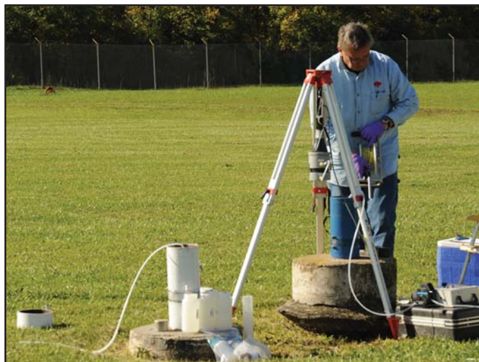
Measuring the water levels in a monitoring well during environmental sampling at NFSS
