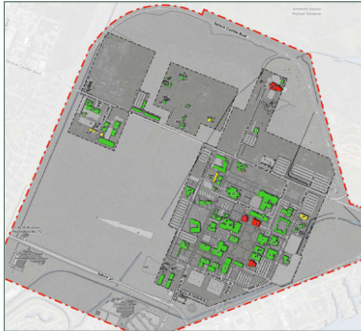
Most JSC structures today consume more than 20 kilowatt-hours per square foot per year. This energy use intensity map shows that by adopting Best Case recommendations, most buildings consume less than 16 kilowatt-hours a year after 20 years (shown in green).
