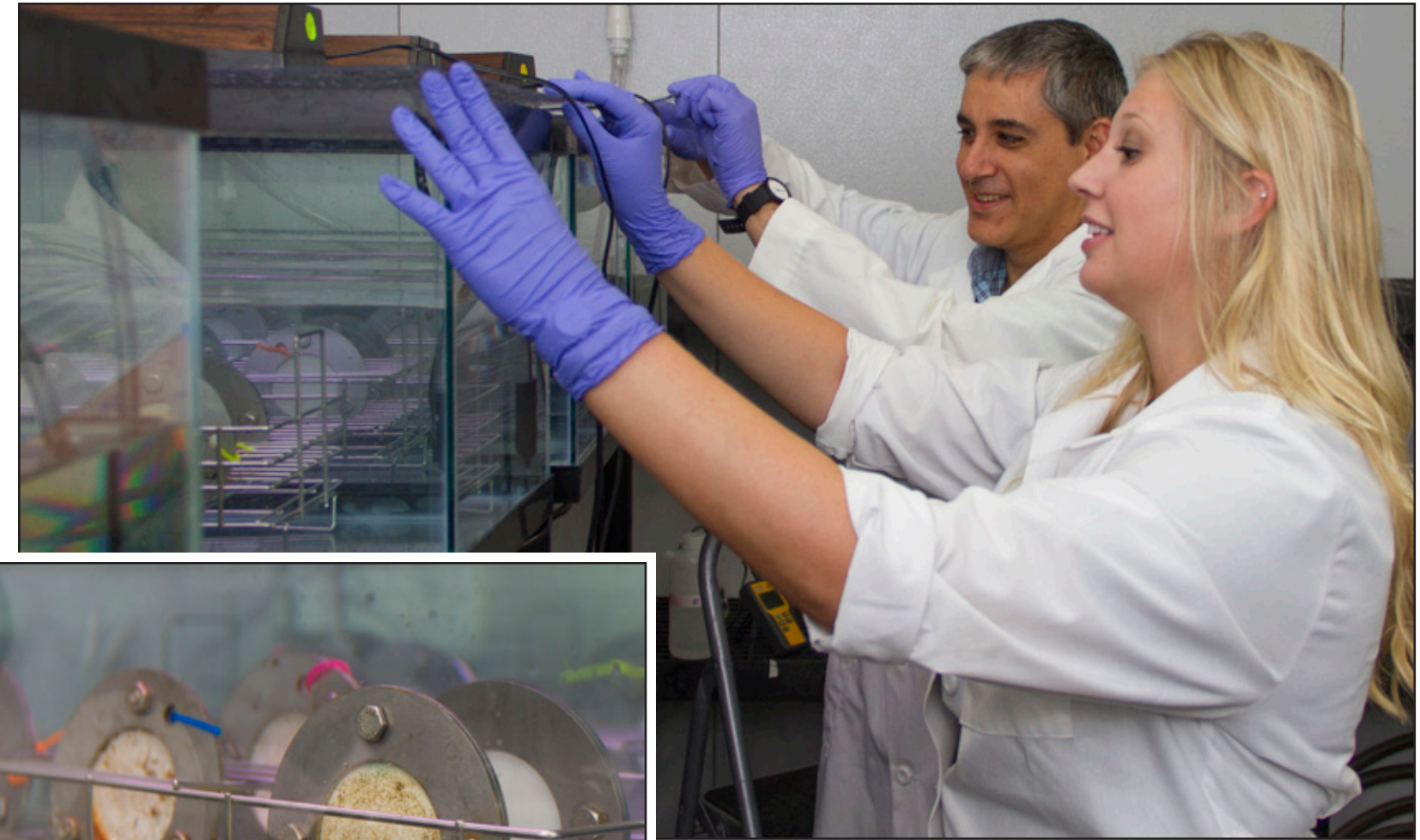
ERDC-EL Research Biologists Dr. Guilherme Lotufo and Lauren Rabalais set up a replicate aquaria experiment in an Environmental Risk Assessment Branch laboratory. They are investigating how increasing degrees of biofouling impacts the uptake rate of munitions constituents using polar organic chemical integrative samplers (POCIS) in coastal environments. Left is a close-up showing POCIS with increasing degrees of biofouling. (Photos by Oscar Reihsmann)
