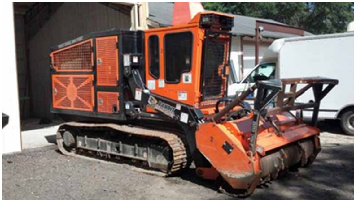
The Bandit, a remote controlled vegetation mulcher, improves and speeds range clearance operations.
