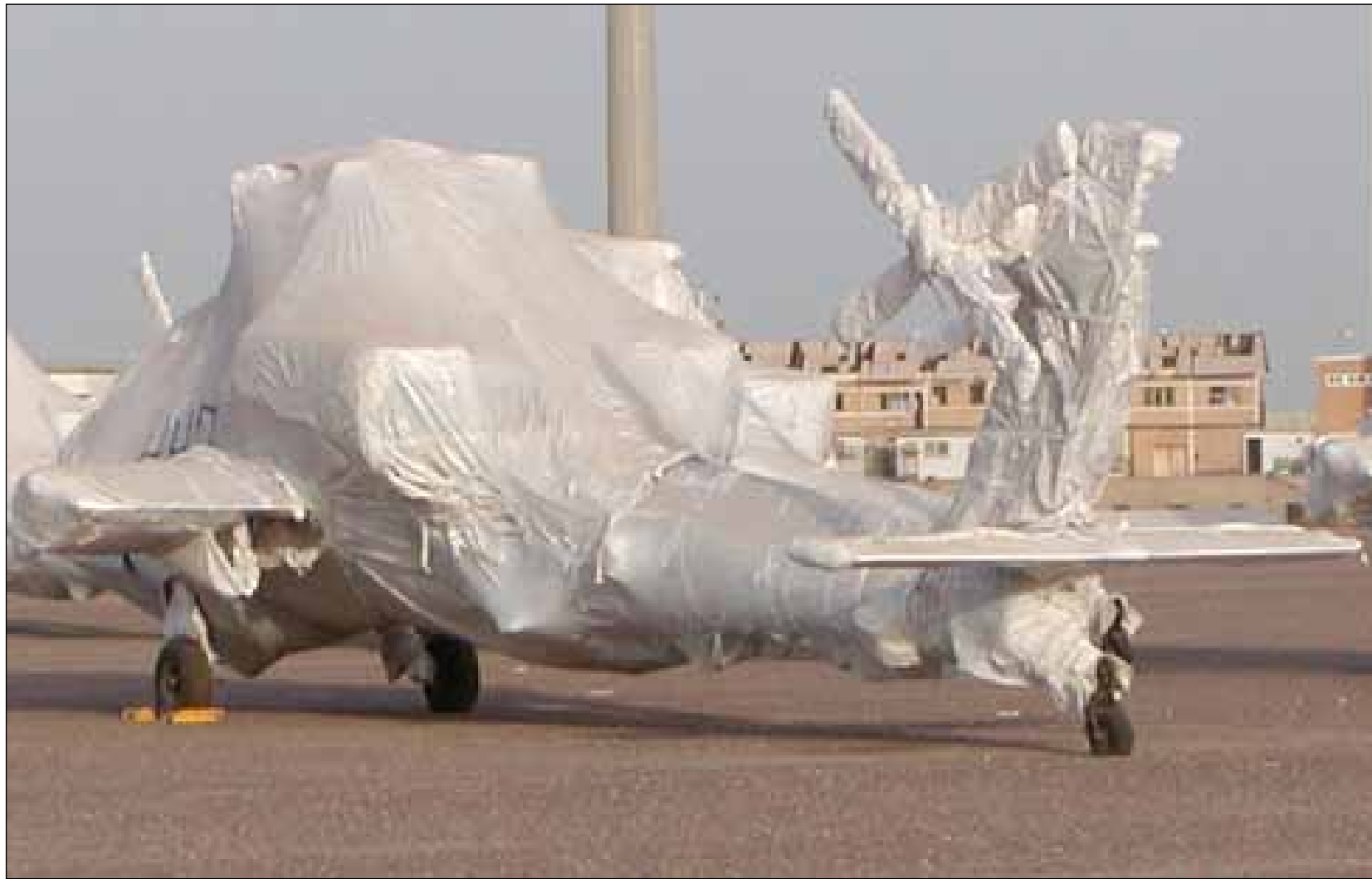
A shrink-wrapped helicopter sits at a loading facility just south of Kuwait City in Kuwait. The shrink wrap on the helicopter helps protect the helicopter and prevent dust and invasive species from entering the equipment once it has been cleaned. (Photo by Al Cofrancesco)
