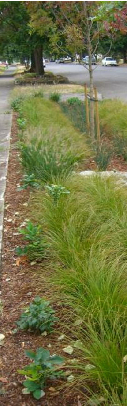
A green street project in Portland absorbs and filters stormwater.
