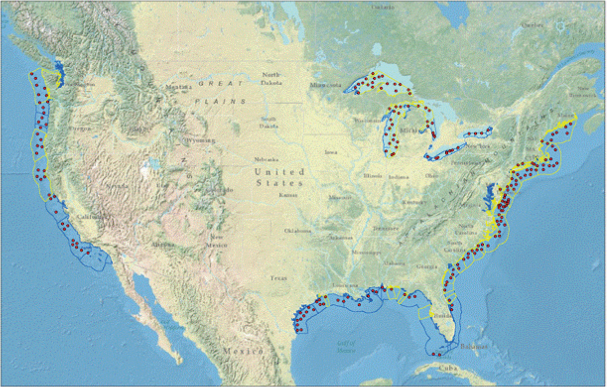
Figure 3-3. Map of 209 selected potential offshore wind projects (red circles) along with ReEDS zones with (yellow) and without (blue) capacity targets
