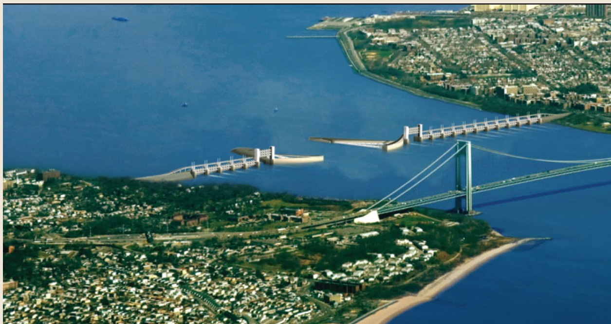
Figure 16.8. Conceptual design of a storm surge barrier in New York City. (Figure source: Jansen and Dircke 2009).
