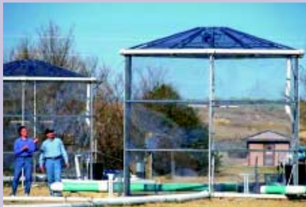
Open-top CO 2 enrichment chambers on the shortgrass steppe in north-eastern Colorado.
