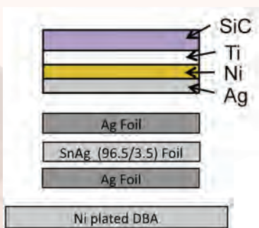
Figure 9.5. Cross-section of various layers in the lead-free 400°C Ag-Sn TLP die attach developed and patented for the high-temperature SiC power module.
