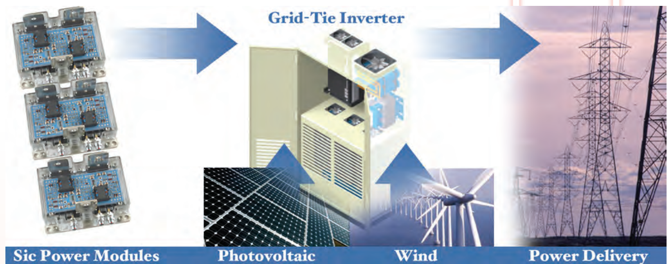
Figure 11.2. The SiC power module's high-energy efficiency and lightweight makes it an excellent choice for use in renewable energy power inverter applications.
