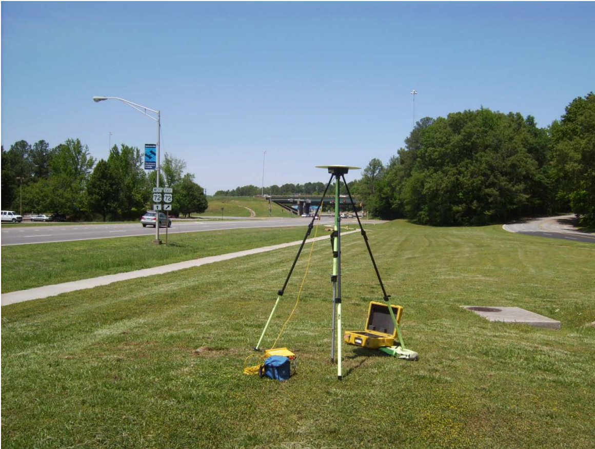
Figure 6-3 Sample Picture of Horizon Showing a Typical GPS Equipment Setup (COE 1 – GPS PROSPECT Class)
