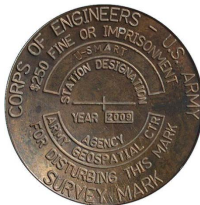
Figure 3-6. Standard brass survey disk
