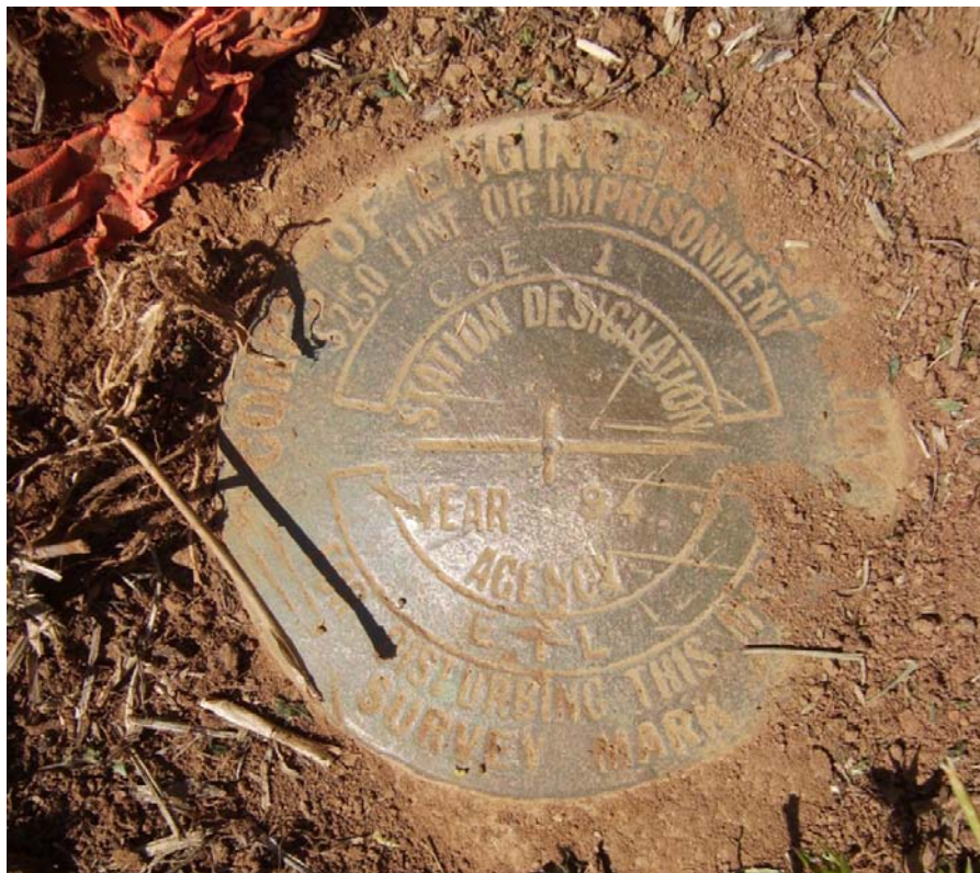
Figure 6-2 Typical Close-Up Picture of a Survey Monument (COE 1 – GPS PROSPECT Class)
