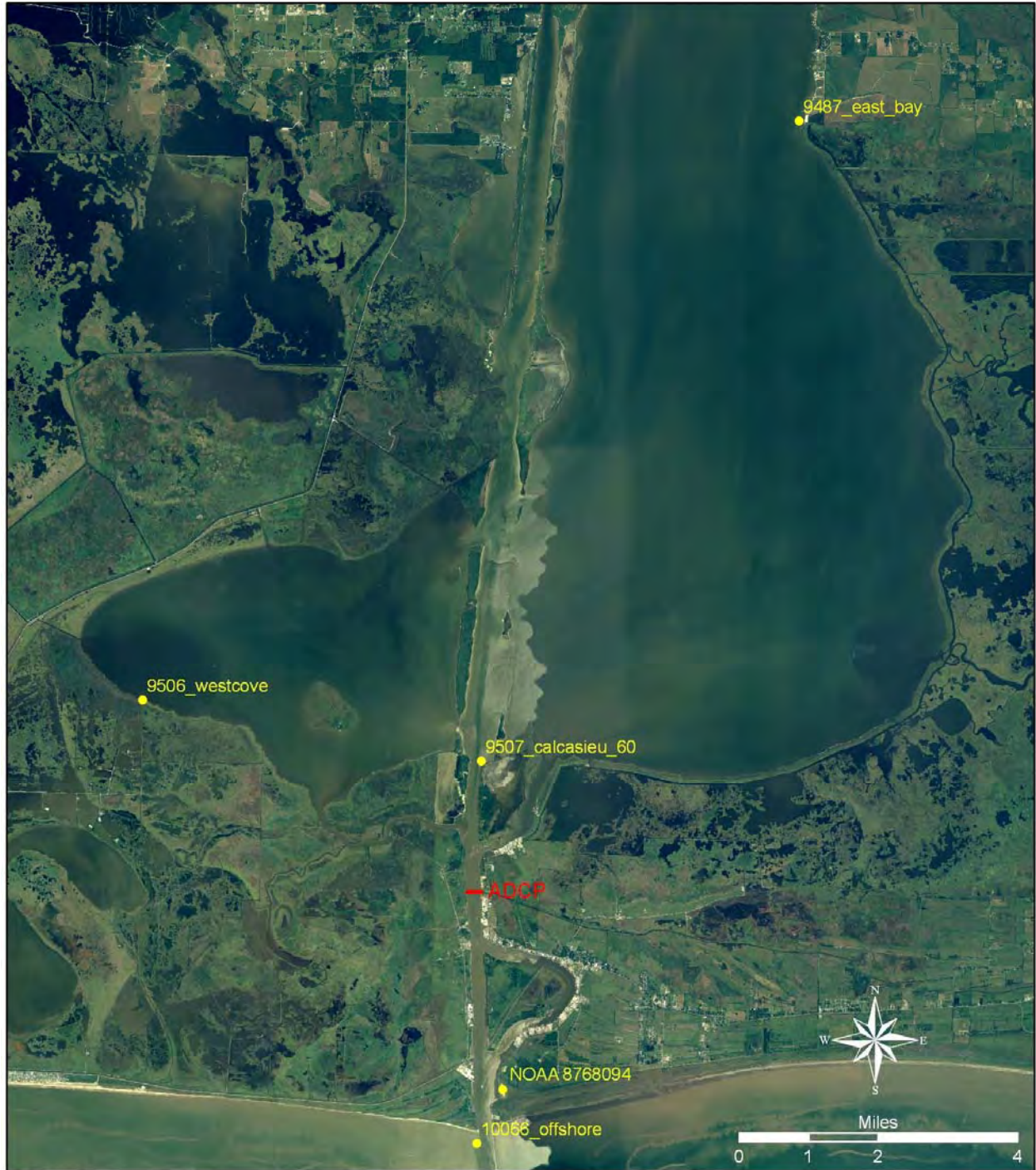
Figure III-2. Tide gage and ADCP transect locations in the southern portion of Lake Calcasieu. Yellow points are tide gage locations and red is the ADCP transect location.
