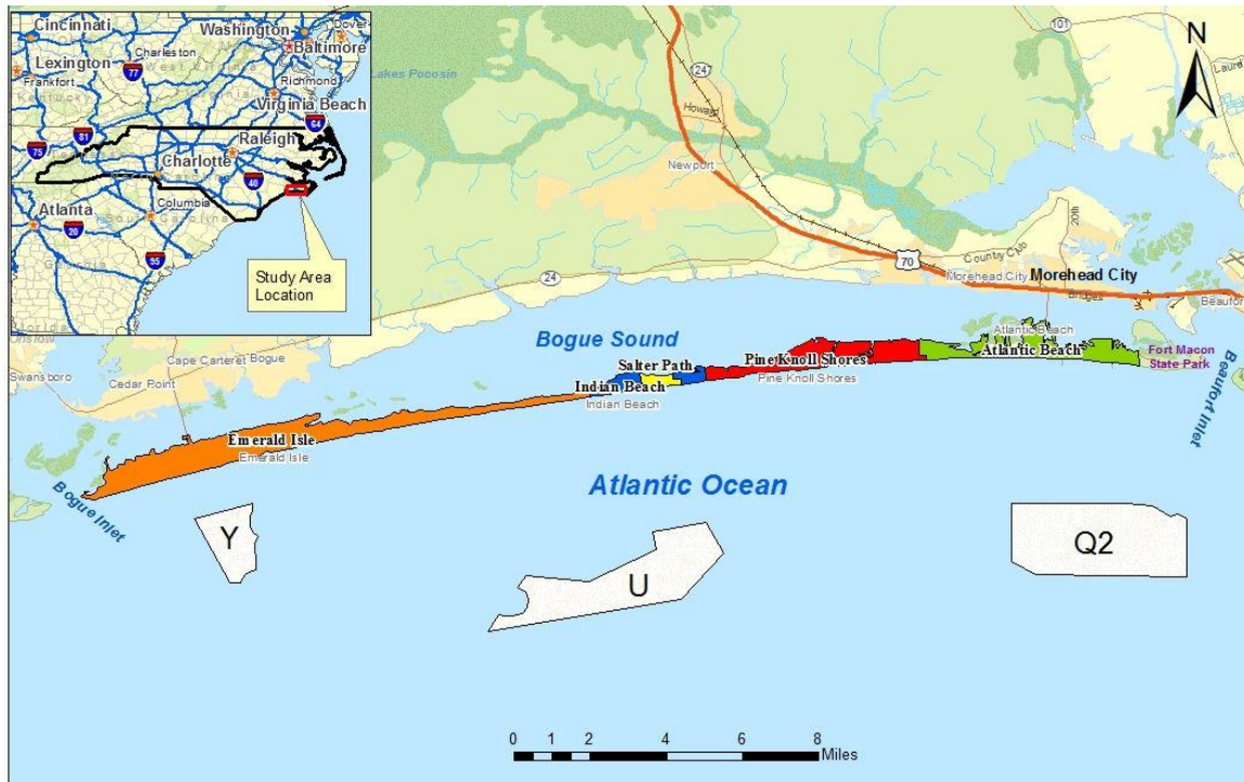
Figure 1: Offshore borrow areas outlined in the Feasibility Study and currently permitted nearshore placement area.
