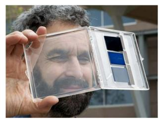
NREL Research Fellow Howard Branz examines silicon wafers with various antireflective treatments. The cells use the NREL black silicon method (top), a conventional antireflective coating with texturing (center), and the conventional texturing method only (bottom).
