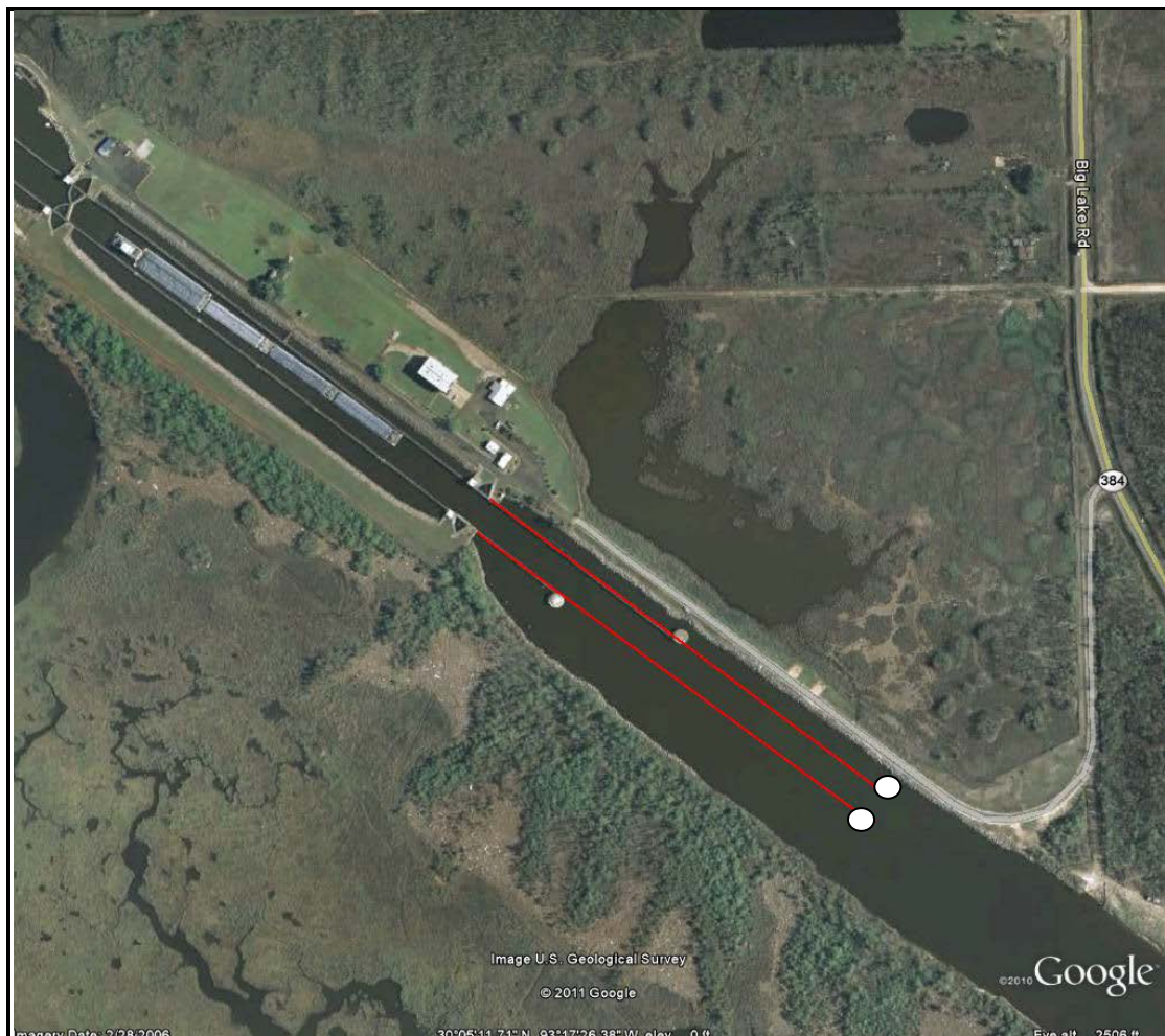
Figure 16. Measure ELB Showing Potential Guide Wall Extensions
