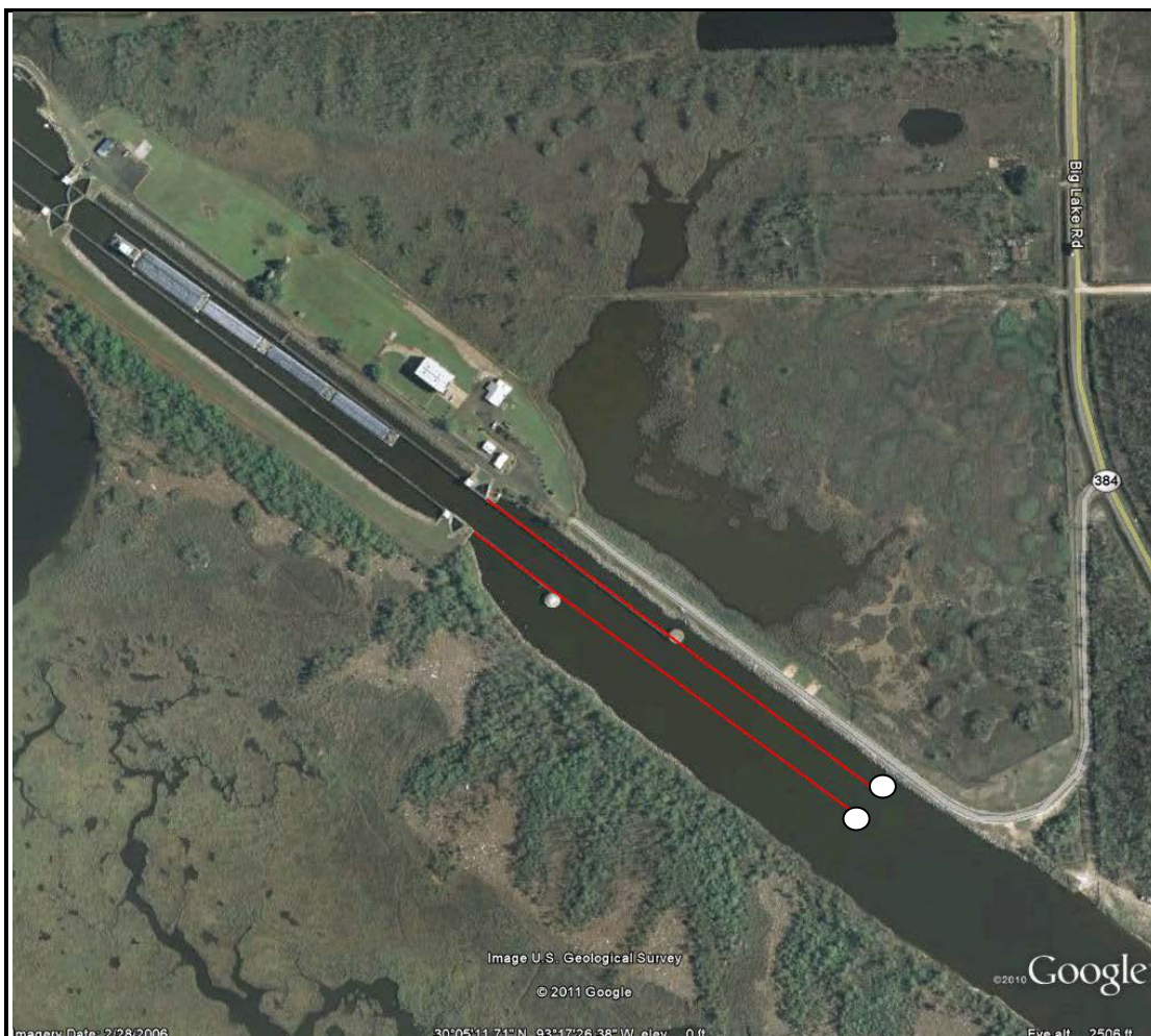
Figure 16. Measure ELB Showing Potential Guide Wall Extensions
