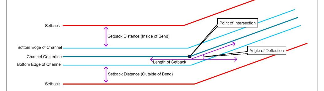
Bend setbacks are based on the angle of deflection of the centerline of the AlVWV channel. The width and length of the setbacks are based on how sharp the turn or bend is. The length of the setback is measured down the channel along the centerline starting at the bend. The width is measured from the near edge of the channel.
