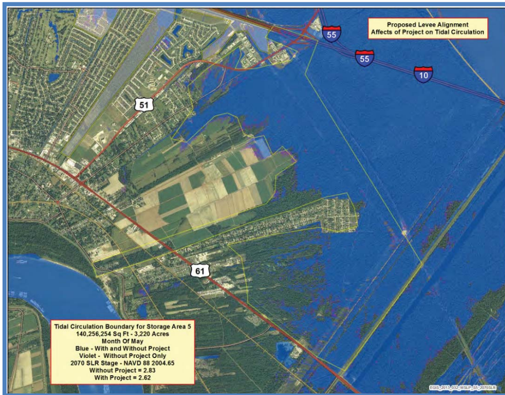
Figure 4-1: Model results of with and without proposed levee alignment affects on tidal circulation.
