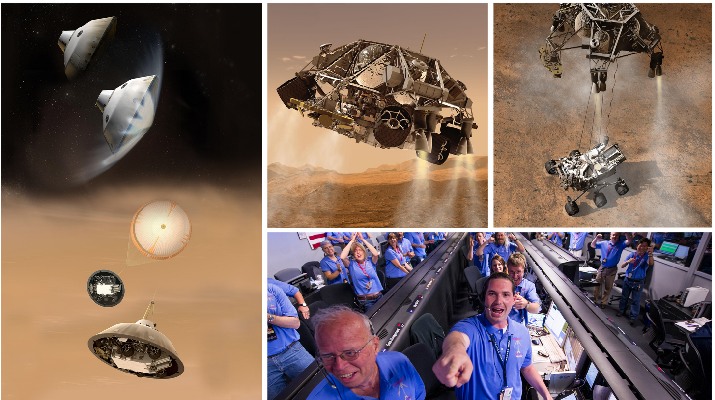
The above sequence depicts the entry, descent, and landing (EDL) phase of the Mars Science Laboratory mission. Instead of the familiar airbag landing systems of the past Mars missions, Mars Science Laboratory used a guided entry and a Sky Crane touchdown system to land the massive Curiosity rover. JPL's mission control room burst into celebration after receiving confirmation of the successful landing.
