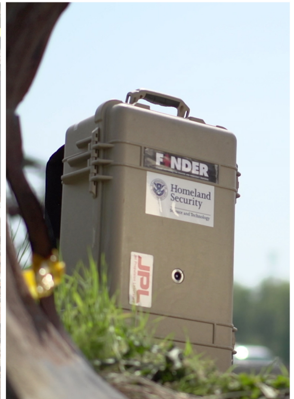
JPL's Finding Individuals for Disaster and Emergency Response (FINDER) prototype technology can locate individuals buried under rubble in disaster scenarios. The suitcase-sized device helped uncover four survivors following the 7.8-magnitude earthquake that devastated Nepal on April 25, 2015.
