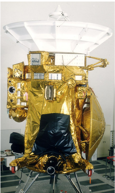
Left: The Cassini spacecraft inside a JPL assembly room. The Cassini orbiter and its two onboard cameras were designed, developed and assembled at JPL. Right: Of the countless equinoxes Saturn has seen since the birth of the solar system, this one, captured here in a mosaic of light and dark, is the first witnessed up close by an emissary from Earth ... none other than our faithful robotic explorer, Cassini.
