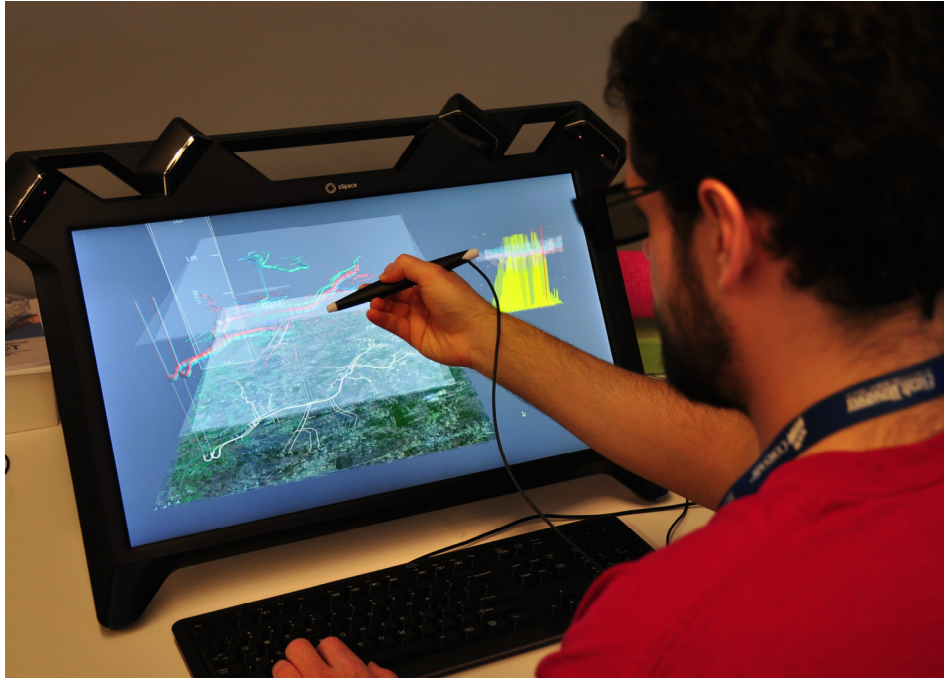
Figure 17. Three-dimensional analysis of the feeder simulation results on a zSpace immersive desktop
