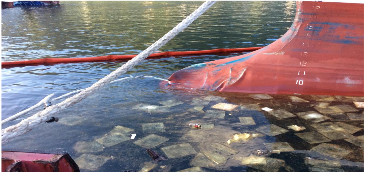
(Pictured: Collision area on bulbous bow of CAPT VINCENT GANN, boom and absorbent pads deployed.)
