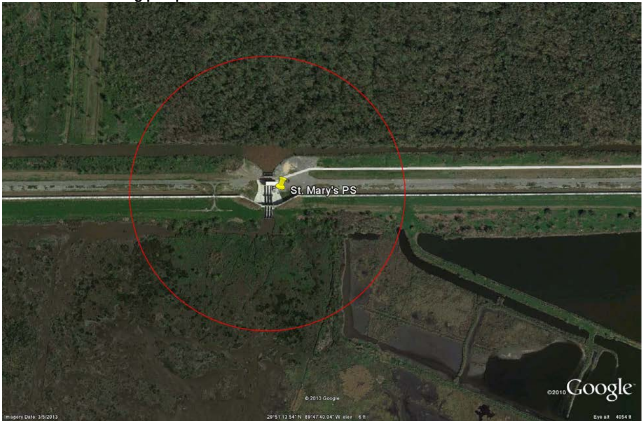
Figure 6: Range of noise impacts illustrated by red circle illustrating 1000 feet surrounding pump station
