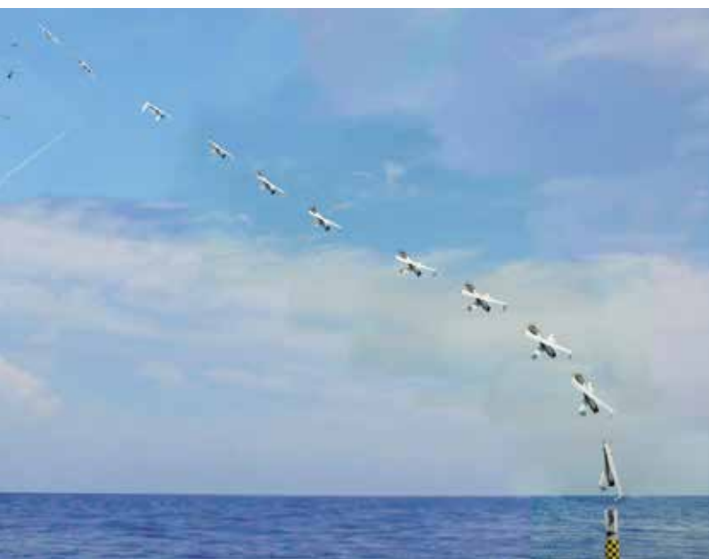
This timelapse photo shows the NRL-developed eXperimental Fuel Cell Unmanned Aerial System (XFC UAS) being deployed. The XFC is a submarine-launched, fully autonomous electric UAS for low-cost ISR missions.
