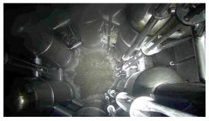
The inside of the test vessel contains six pulse jet mixers used to keep the solids suspended in the simulated radioactive waste. More images available at <a href="http://bit.ly/2iB4FpW">http://bit.ly/2iB4FpW</a>.
