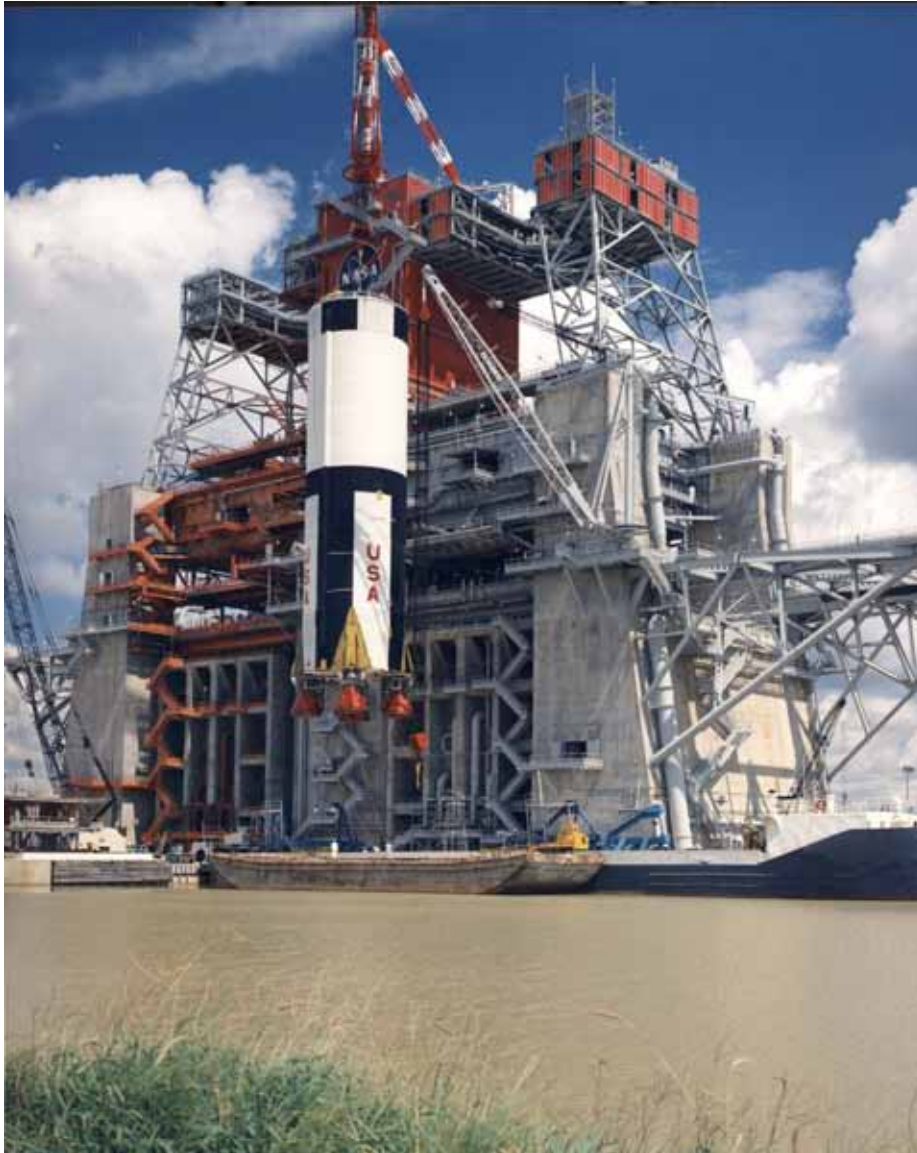
The first stage of the huge Apollo Saturn V moon rocket is lifted by crane for installation into the B-2 test stand at the Mississippi Test Facility, 1967.
