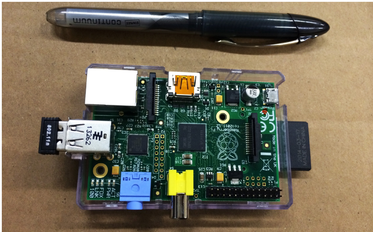
Raspberry Pi, a computer the size of an iPhone, can hold a year's worth of weather information collected from a 3-D-printed station. Photo: Heather Freitag, USAID.
