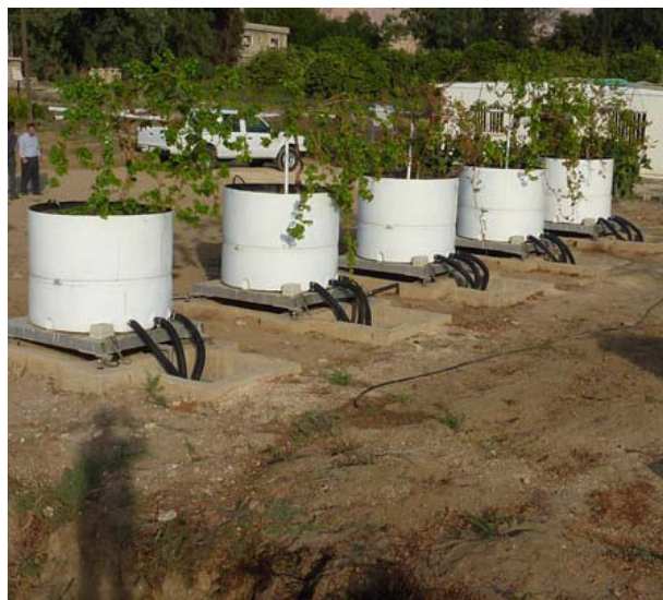
Lysimeter experiments in Jordan used by MERC scientists to minimize agricultural water use requirements. Photo: Dr. Alon Ben Gal.
