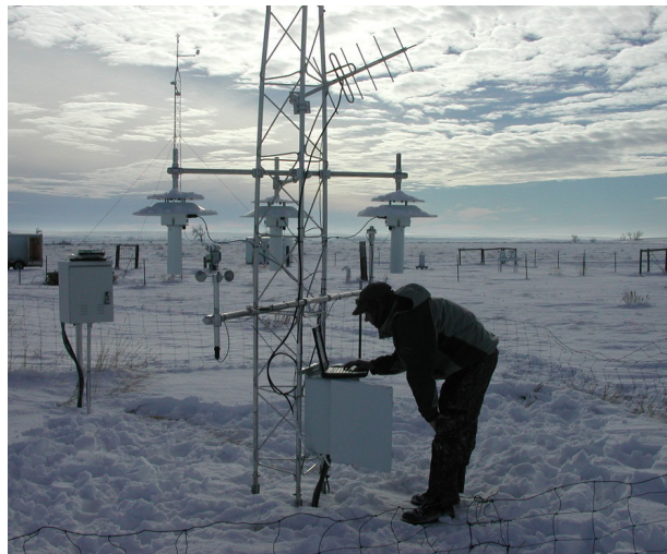
An Air Resources Laboratory engineer works on a U.S. Climate Reference Network (USCRN) site in Wolf Point, MT. The USCRN is a systematic and sustained network of climate monitoring stations with sites across the conterminous U.S., Alaska, and Hawaii that provide a continuous series of climate observations like temperature, precipitation, wind speed, and soil conditions.
