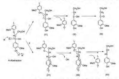
Typical thermal depolymerization reactions at relatively high temperature
