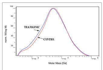
FIGURE 8 | Molecular weight distribution curves of acetylated lignin isolated from the wild-type and COMT transgenic switchgrass.
