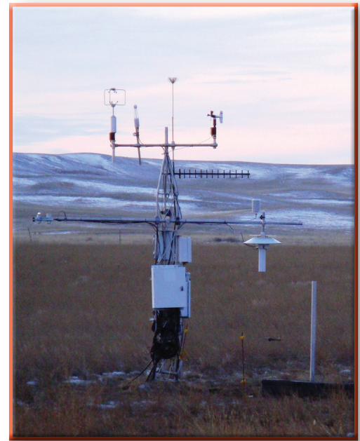
A Surface Energy Budget station at Ft. Peck, MT (Photo: NOAA)
