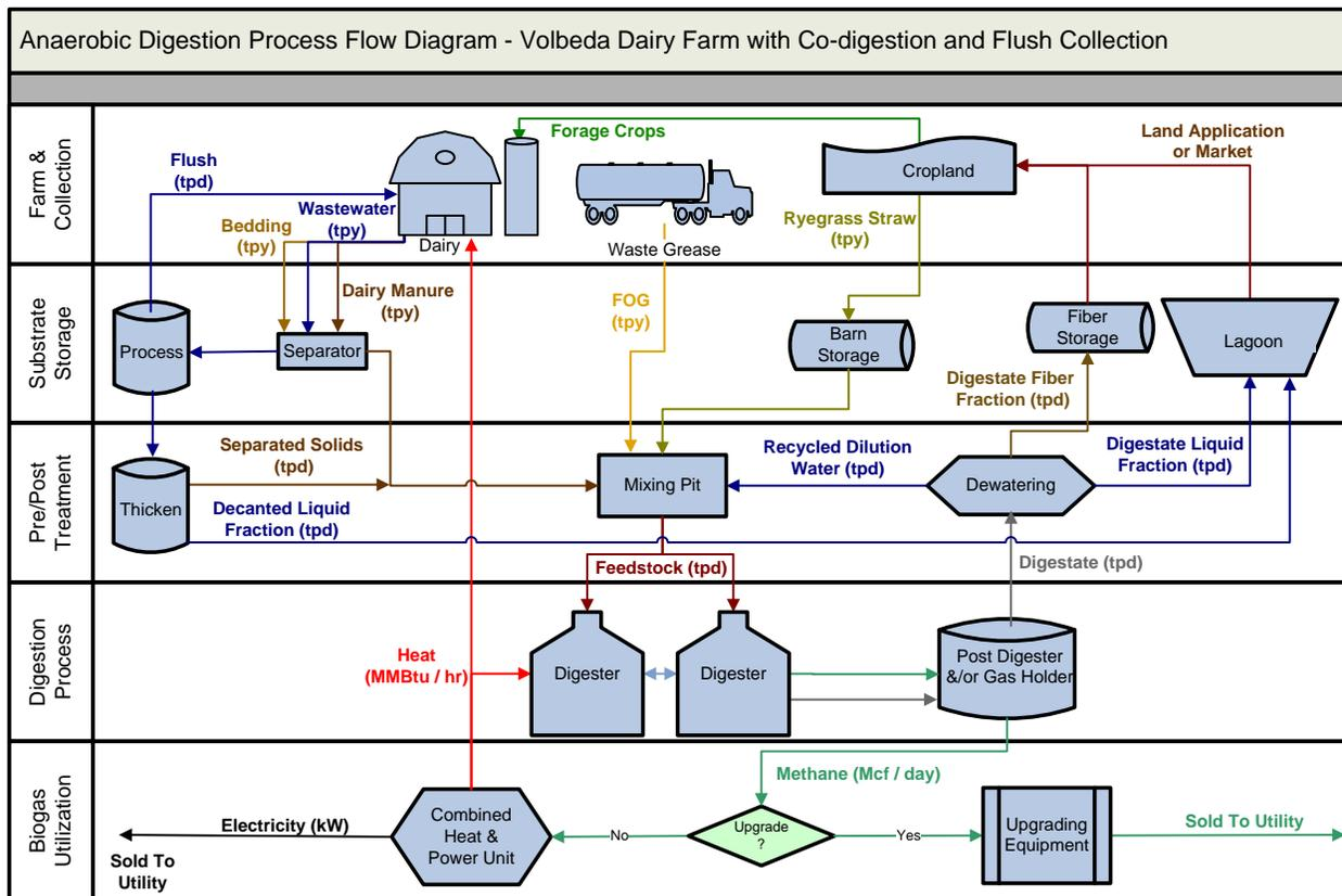
Figure 7 Process flow diagram of potential on-farm biogas plant with co-digestion (EC Oregon, 2009)
