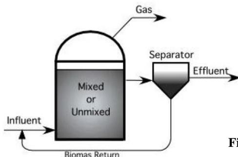
Figure 12 Contact reactor (Burke, 2001)
