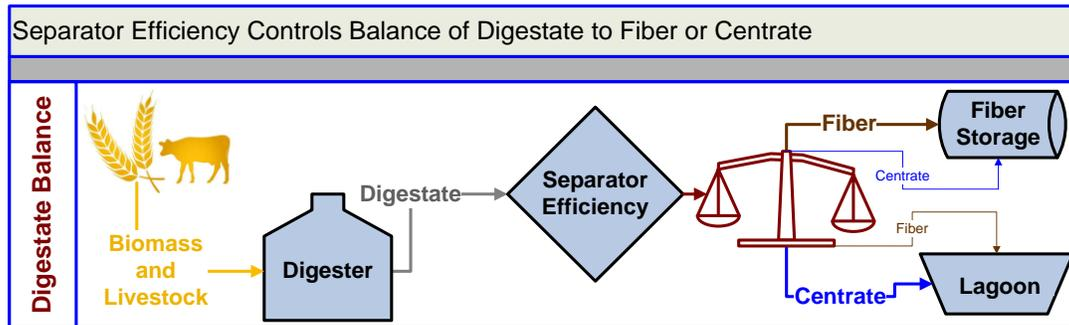
Figure 20 Separator efficiency and digestate balance (EC Oregon, 2009)
