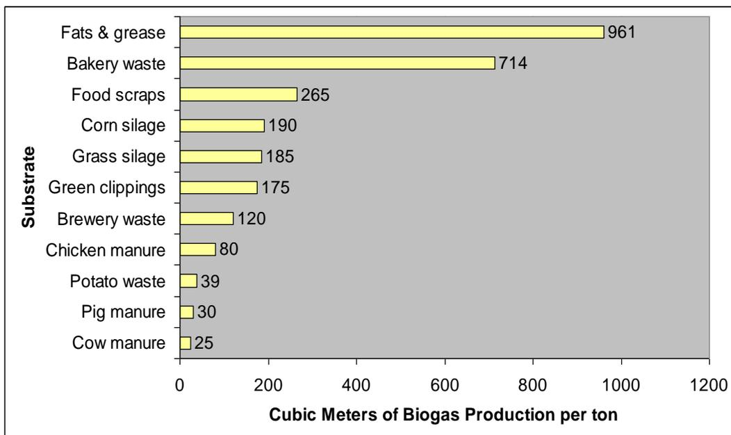
Figure 14 Cubic meters of biogas production per ton of substrate (Redrawn from Kramer, 2008)
