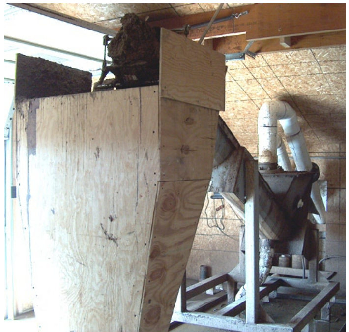
Solid/liquid manure separator with chute to direct solids to the storage bay below
