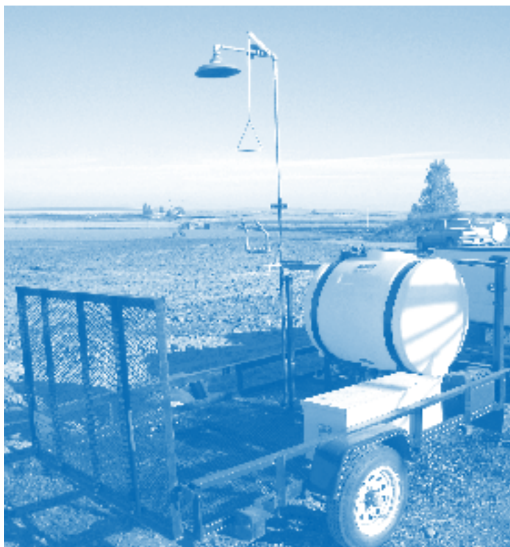
Portable decontamination unit
