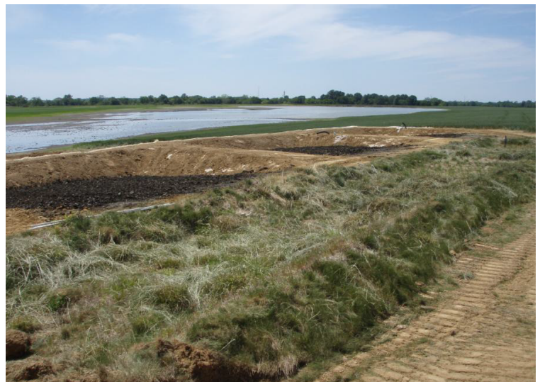
Research plots for the Maryland Port Administration Cox Creek dredge study will determine if dredge sediment is suitable for reuse.
